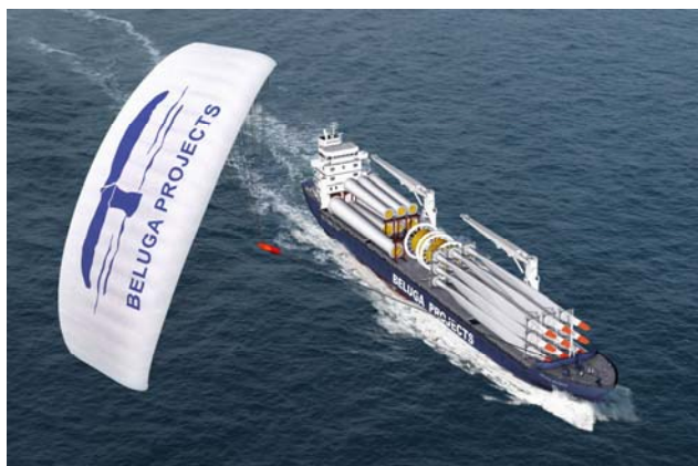
Fig.8: Towing kite harnessing wind energy, source: www.skysails.de
